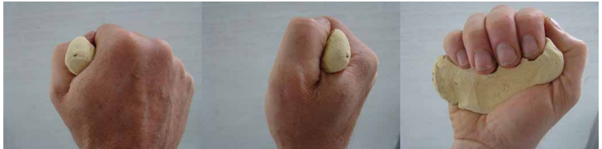
zeeklei, handvorm gestookt op 1060 graden
